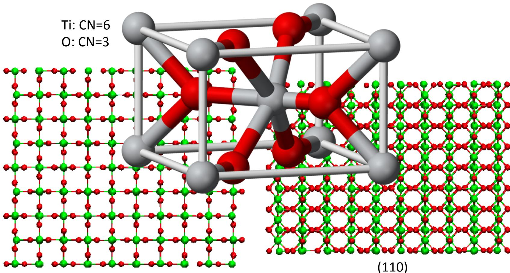
[1] Rutile primitive tetragonal unit cell, with unit cell parameters  $a=4.587\text{\AA}$ , and  $c=2.953\text{\AA}$ .
