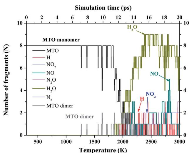
Fig. 2 Species analysis for the decomposition of **P2<sub>(1)</sub>-MTO** heated from 300 to 3000 K over 20 ps. During 7 to 11 ps, H transfer occurs and at ~11.5 ps ( $T = 1800$  K), the first H<sub>2</sub>O released. Starting at 13 ps (~2050 K), one NO molecule is released. The main product of **MTO** decomposition is H<sub>2</sub>O.
