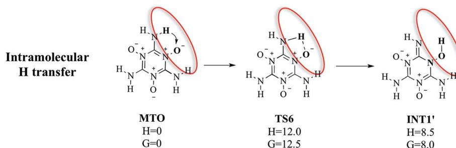
Fig. 5 The reaction mechanism for the intramolecular H transfer path **MTO-TS6-INT1'** that forms one molecule of **INT1**, this path was observed in gas phase but was not observed in the DFT-MD simulations. Here energies are in  $\text{kcal mol}^{-1}$ .
