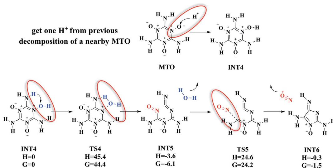
Fig. 4 The mechanism of our proposed pathway for the reactions releasing H<sub>2</sub>O and NO<sup>+</sup> from MTO, which starts with an H<sup>+</sup> transfer from a previously decomposed MTO molecule to an oxygen atom (see the red lines in Fig. 2, which indicate dissociated H atoms) of an unreacted MTO to form INT4. Then INT4 releases one H<sub>2</sub>O to form INT5, which is followed quickly by NO<sup>+</sup> release to form INT6. Units are in kcal mol<sup>-1</sup>.
