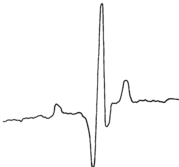
FIG. 1. The J=1 \rightarrow 2 transitions of NO^+ . Frequency increases from right to left.
