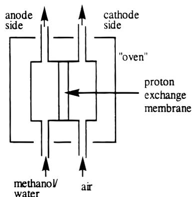
Figure 1. Schematic of a direct methanol fuel cell.
