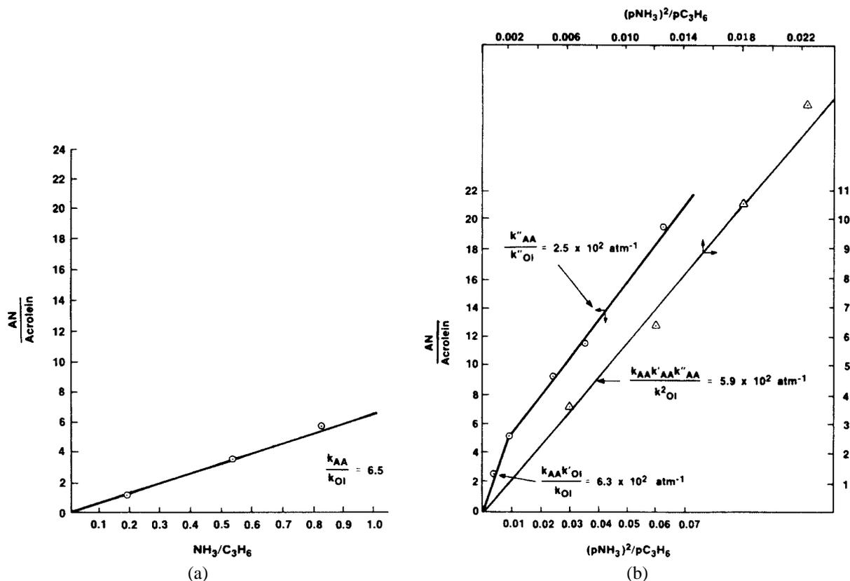
Figure 9. Relationship between the ammonia/propene feed ratio and the acrylonitrile/acrolein product ratio. This depends on the partial pressure of reactants in the feed. (a) Low feed pressure ( $p(\text{C}_3\text{H}_6) = 0.041$  atm) and (b) intermediate feed pressure ( $p(\text{C}_3\text{H}_6) = 0.082$  atm; dual-slope line) and high feed pressure ( $p(\text{C}_3\text{H}_6) = 0.14$  atm; single-slope line). Burrington, Kartisek and Grasselli [52].
