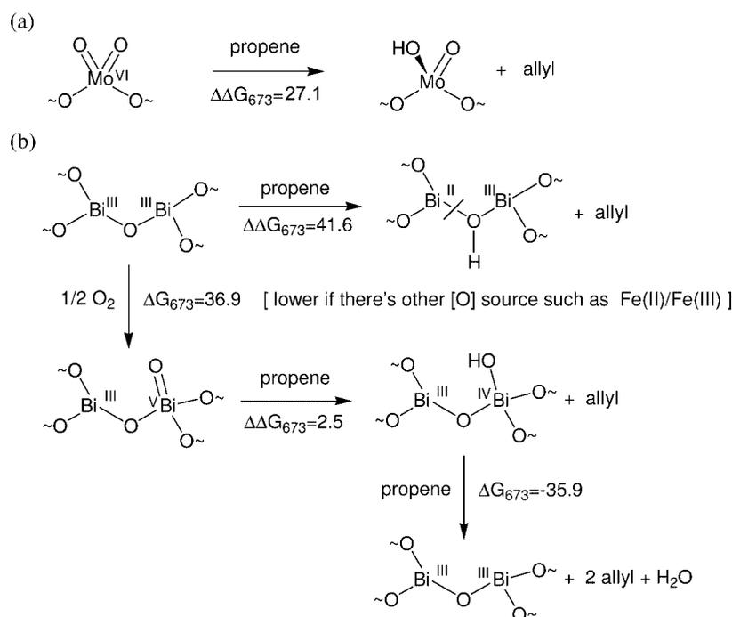
Scheme 2. Summary of the H abstraction from propene by (a) the molybdenum site (implausible) and (b) the bismuth site (plausible only on the oxidized site, which is likely consumed very quickly).
