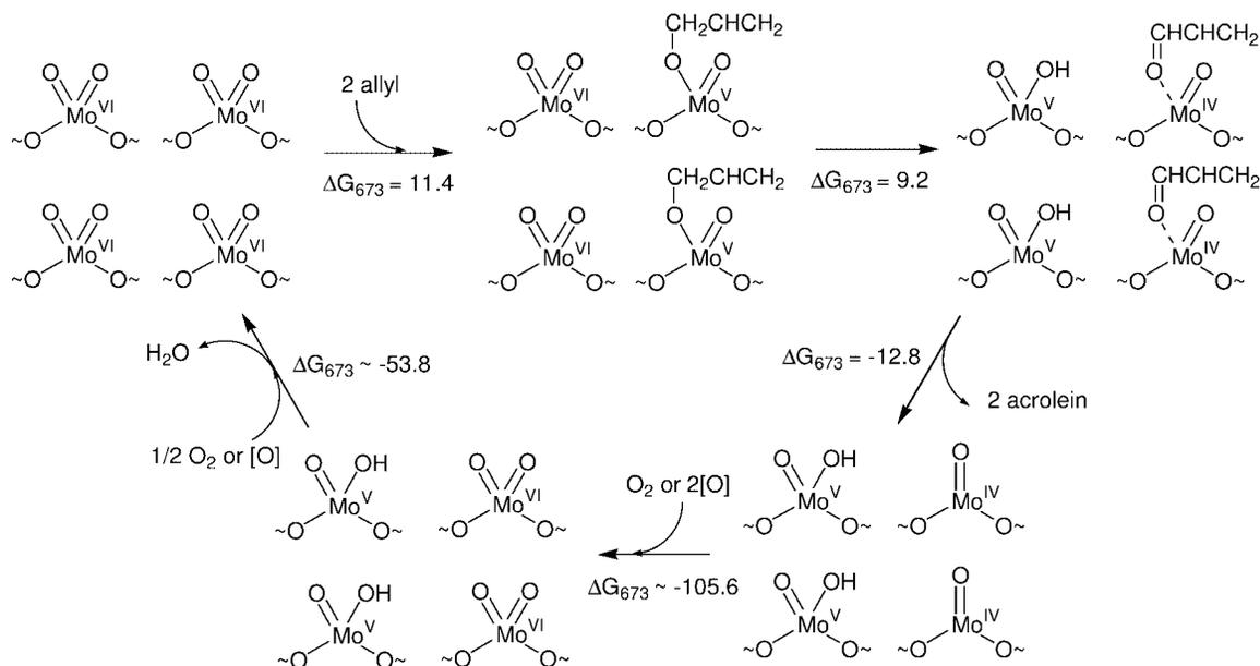
Scheme 5. Oxidation part 2. Allyl adsorption, oxygen insertion, and reoxidation on molybdenum site.
