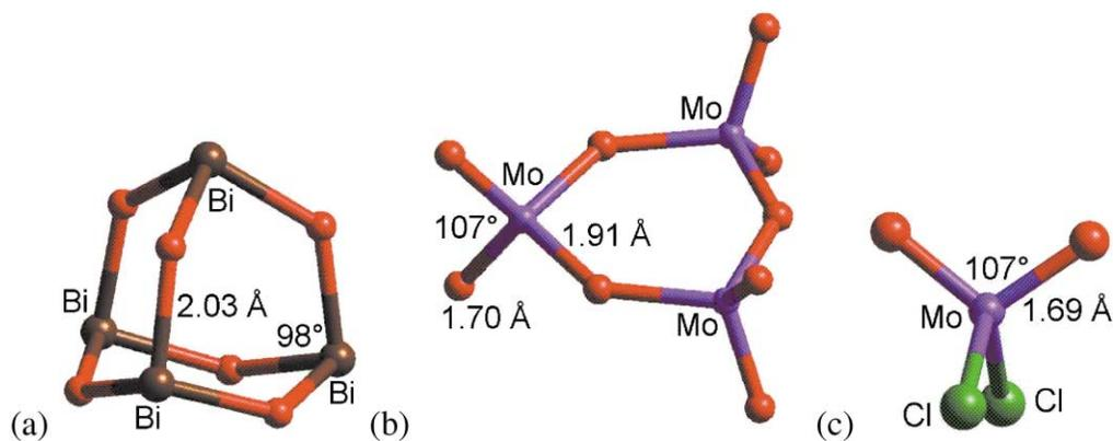
Figure 2. Model clusters used to represent (a) the bismuth site (Bi<sub>4</sub>O<sub>6</sub>) and (b) the molybdenum site (Mo<sub>3</sub>O<sub>9</sub>). (c) Smaller model cluster used to represent the molybdenum site instead of (b) in the later part of the work.
