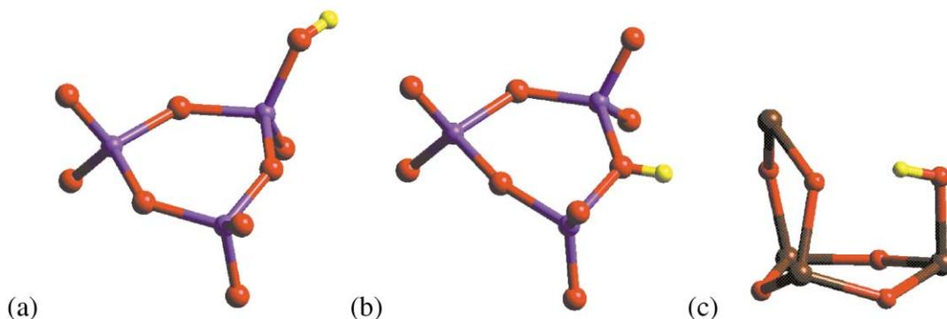
Figure 3. Optimized structures showing a hydrogen adsorbed on (a) an oxo group of Mo<sub>3</sub>O<sub>9</sub>, (b) a bridging oxygen of Mo<sub>3</sub>O<sub>9</sub>, and (c) on an oxygen of Bi<sub>4</sub>O<sub>6</sub>.
