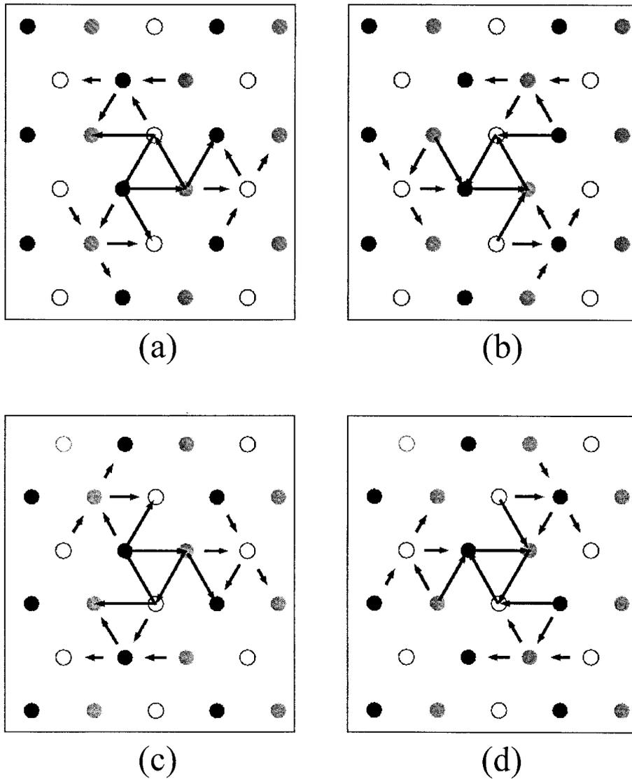
Figure 1. Differential displacement (DD) maps of the equilibrated dislocation core structures. Figure (a) and (b) show two types of core configurations of the dislocation with  $b = a/2[111]$ , while Figure (c) and (d) show core configurations of the dislocation with  $b = a/2[-1-1-1]$ .
