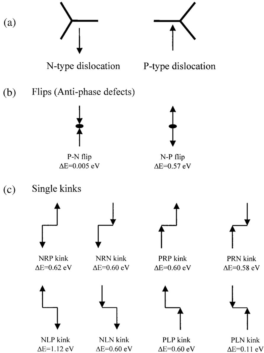
Figure 3. (a) Schematic drawings of N-type dislocation core and P-type dislocation core. Arrows indicate whether three central columns of atoms move inward or outward defect (flip or kink) region. (b) Sketches and formation energies of the flips. (c) Sketches and formation energies of the isolated single kinks.
