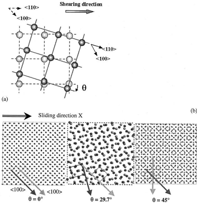
FIG. 2. (a) Schematic diagram showing the lattice mismatch of Ni(100) interfaces. (b) The  $z$  projection of the simulation cell. The dark circles are atoms of upper slab and light circles are atoms of lower slab.  $\theta$  is the lattice misorientation angle between the upper and lower slabs. The sliding direction is along the  $x$  direction of the simulation cell.
