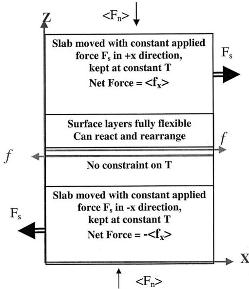
FIG. 1. Projection along the  $y$  direction of the 2D periodic cell (along the  $x$  and  $y$  directions) for the steady-state nonequilibrium molecular dynamics simulations.  $F_s$  is the applied external force on two moving slabs with 12 layers of atoms,  $f$  is the frictional force during the sliding of two slabs, and  $\langle F_n \rangle$  is the normal load in the  $z$  direction.
