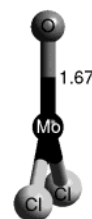
Figure 7. Model cluster MoOCl 2 representing the reduced molybdenum site Mo(IV). Mo=O bond length is shown together in Å.
