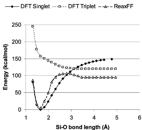
Figure 5. Dissociation of the Si-O bond in H<sub>3</sub>Si-O-SiH<sub>3</sub>.
