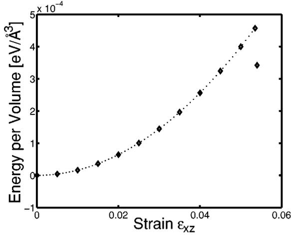
FIG. 4. Energy versus strain of vanadium in a quadrupolar cell of size  $42 \text{ \AA} \times 20 \text{ \AA}$ . Diamonds denote the energy calculated at various strains. The dotted line is a quadratic fit up to the Peierls stress.
