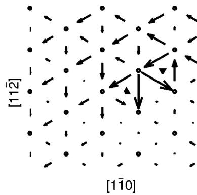
FIG. 9. Differential displacement map at an applied strain of 0.05 ( $\sigma_{xz}=1.76$  GPa). The cell has converged to within the tolerance defined in the text. This figure shows that the core has moved from the old triad (solid upright triangle) to a new triad (upside-down triangle) along a  $\langle 112 \rangle$  direction.
