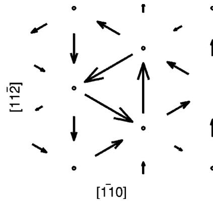
FIG. 6. Easy-core structure for tantalum calculated within density- functional theory. This cell of size 41 Å × 20 Å gives very similar results to the cell of size 23 Å × 12 Å, used in Ref. 19.
