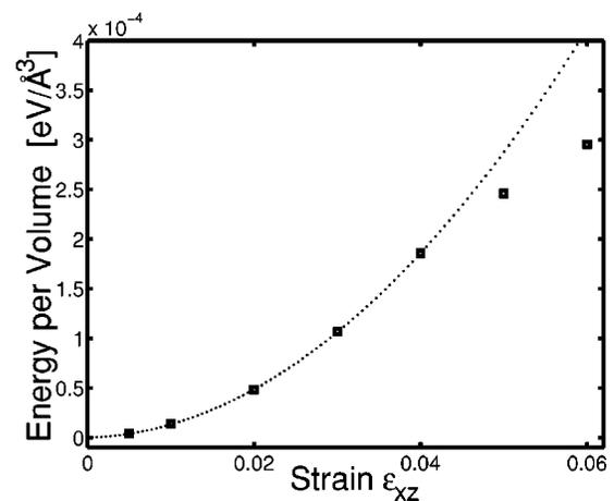
FIG. 7. Energy versus strain for tantalum in a cell of size 23 Å × 12 Å, calculated within density-functional theory. Squares denote the calculate energy at various strains. The line is a quadratic fit to the first five data points. The graph indicates that the points with strain at and above 0.05 ( $\sigma_{xz} = 1.76$  GPa) will be at a stress above the Peierls stress.
