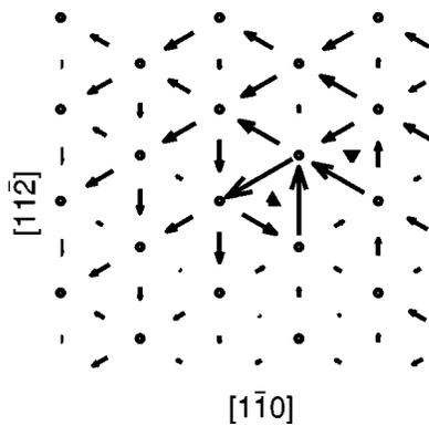
FIG. 8. Differential displacement map at an applied strain of 0.04 ( $\sigma_{xz}=1.41$  GPa). The cell has converged to within the tolerance defined in the text. The solid upright triangle is the location of the center of the dislocation, under no stress. The center of the dislocation, at this applied stress, has not moved.
