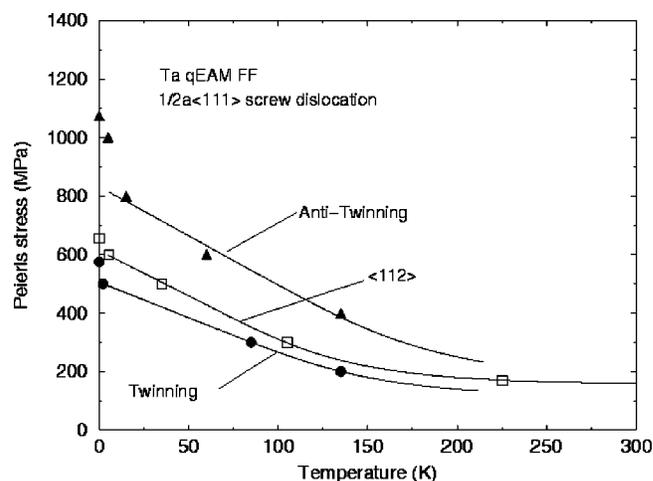
FIG. 2. Temperature dependence of the Peierls stress along various directions: the  $\langle 112 \rangle$ , twinning and antitwinning directions. The fits are done for the high-temperature data using Eq. (1). The temperature is in degrees Kelvin, and the stress in mega-Pascals.
