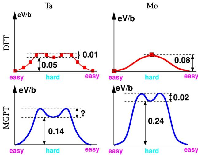
FIG. 5. (Color online) Energy landscape per Burgers vector along a reaction coordinate when going from the easy-core to the hard-core configurations in tantalum and molybdenum: density-functional theory (squares in upper panels) and MGPT (curves in lower panels). *Ab initio* results for molybdenum are from Ref. 19, and the MGPT results for tantalum are from Ref. 11.
