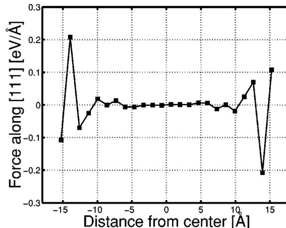
FIG. 1. Force on the atoms, along the [111], due to the presence of a domain boundary. The forces are plotted as a function of distance from the center of the unit cell. The domain boundary is generated such that the nearest-neighbor distance is always within 95% of the bulk ( $\alpha = 1/4$ ).
