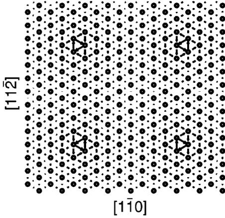
FIG. 3. Quadrupolar unit cell of size  $42 \text{ \AA} \times 41 \text{ \AA}$ : relative displacements of neighboring columns of atoms (arrows) and dislocation centers (triad of arrows). Note, that in the calculations half the amount of such cells are used, which can always be done with an appropriate choice of lattice vectors (Ref. 36).
