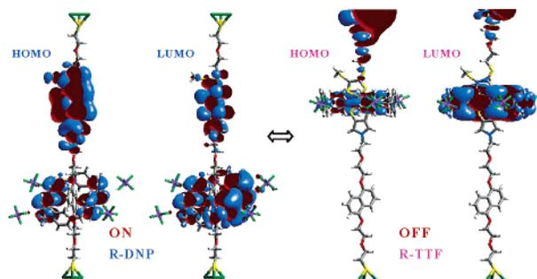
**Figure 2.** MOs of Au-rotaxane-Au switch. Green represents Au atoms, yellow is S, gray is C, red is oxygen, and white is hydrogen. The ring is CBPQT<sup>4+</sup>, with 4 PF<sub>6</sub><sup>-</sup> units around. The TTF and DNP units are located at the top and bottom halves of the dumbbell, respectively. The total is 186 atoms.
