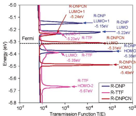
**Figure 3.** Transmission function of rotaxane components. Blue curve is for R-DNP, pink curve is for R-TTF, and red curve is for R-DNPCN. The dashed line is the Fermi energy of Au electrodes,  $-5.31$  eV.
