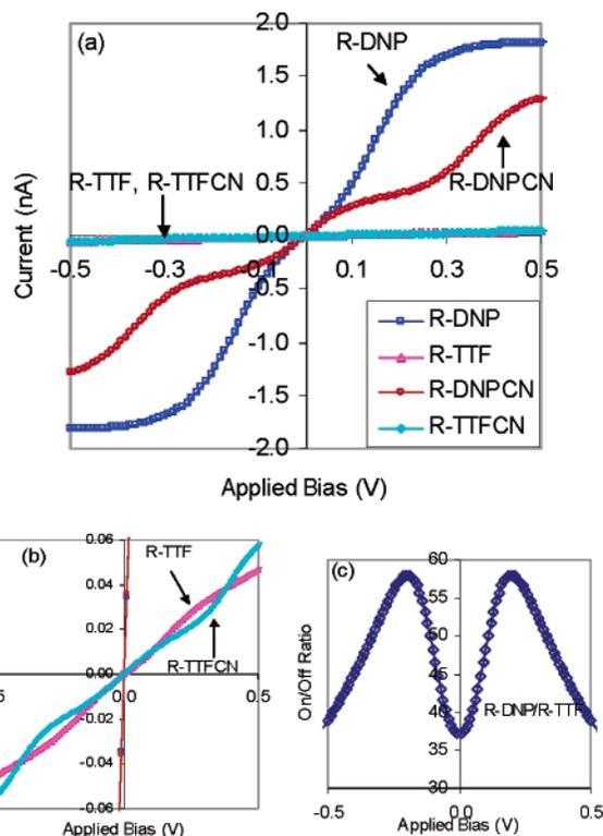
**Figure 1.**  $I$ – $V$  curve of Au–rotaxane–Au switch. (a) The four  $I$ – $V$  curves correspond to ring on DNP (R-DNP), on TTF (R-TTF), and for the modified version of the rotaxane bearing a CN group substituted on the DNP unit, R-DNPCN, and R-TTFCN states. (b) Small-scale  $I$ – $V$  curve of R-TTF and R-TTFCN. (c). The voltage-dependent ON/OFF ratio.
