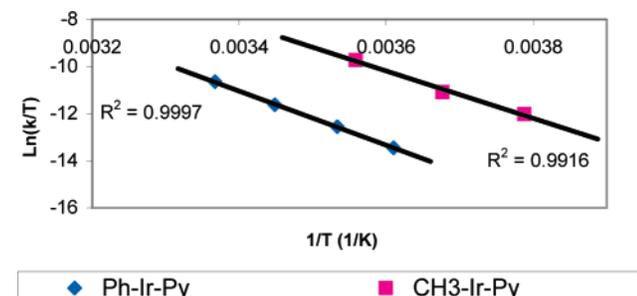
Figure 8. Eyring plot for pyridine exchange with **Ph-Ir-Py** and **CH<sub>3</sub>-Ir-Py**.
