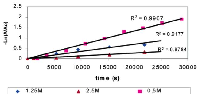
Figure 10. First-order plots for trans-cis isomerization of **Ph-Ir-Py**.
