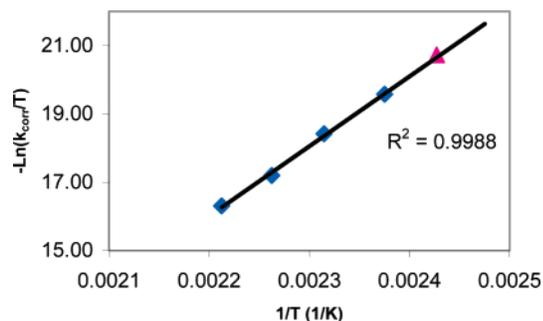
**Figure 15.** Eyring plot for the reaction of  $\text{CH}_3\text{-Ir-Py}$  ( $\blacklozenge$ ) with  $\text{C}_6\text{D}_6$  at  $[\text{Py}]/[\text{C}_6\text{D}_6] = 0.045$ .  $k_{\text{corr}} = k_{\text{obs}} \times [\text{Py}]/[\text{C}_6\text{D}_6]$ . ( $\blacktriangle$ ) =  $\text{PhCH}_2\text{CH}_2\text{-Ir-Py}$ .
