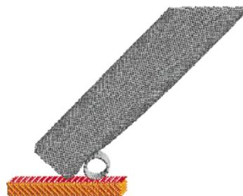
**Figure 8.** A 40,40 SWNT probe imaging a prone 16,16 SWNT at  $\phi = 40^\circ$  showing that this tilt angle is inappropriate because it allows the probe to contact the surface *and* the sample at different horizontal positions *simultaneously*. This type of inappropriate contact causes severe lateral shifting and size distortion of the AFM image, as depicted in Figure 7.
