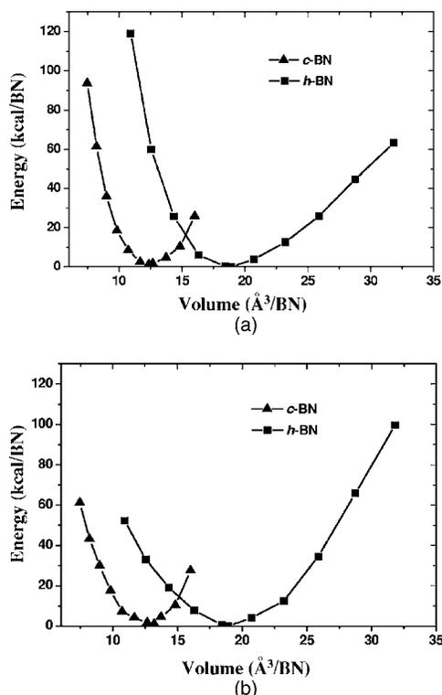
FIG. 5. Equations of states for compression and tension of *h*-BN and *c*-BN crystals, calculated using the (a) PW91 and (b) ReaxFF<sub>HBN</sub> methods.
