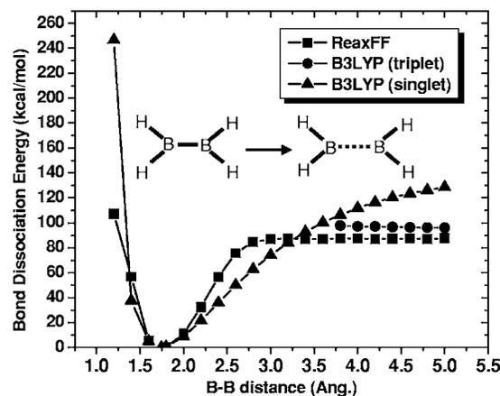
FIG. 1. B3LYP and ReaxFF<sub>HBN</sub> data for dissociation of B–B bond in the H<sub>2</sub>B–BH<sub>2</sub> cluster.
