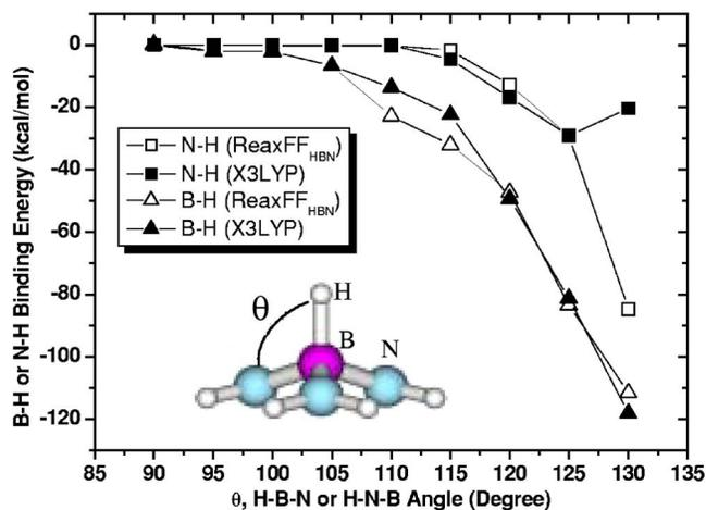
FIG. 3. X3LYP (filled) and ReaxFF<sub>HBN</sub> (opened) results on B–H (triangle) and N–H (square) bond energies in H–B(NH<sub>2</sub>)<sub>3</sub> and H–N(BH<sub>2</sub>)<sub>3</sub> clusters as a function of the out-of-plane angle. The inset displays the H–B–N angle  $\theta$  in the H–B(NH<sub>2</sub>)<sub>3</sub> cluster where red, blue, and white atoms mean boron, nitrogen, and hydrogen, respectively.
