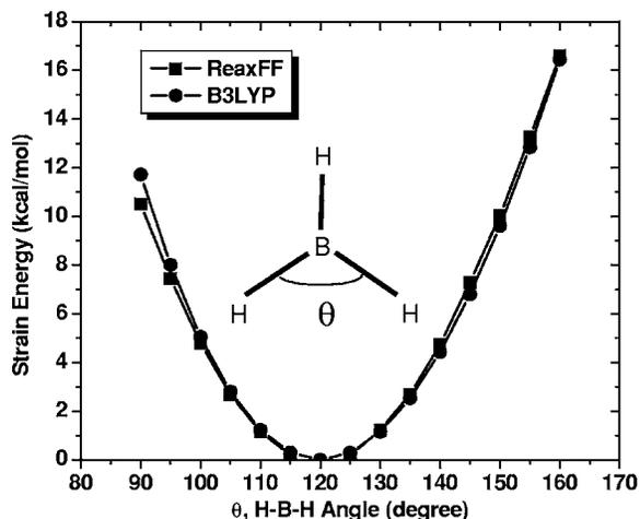
FIG. 2. B3LYP and ReaxFF<sub>HBN</sub> data for angle distortion of H–B–H in the BH<sub>3</sub> cluster.
