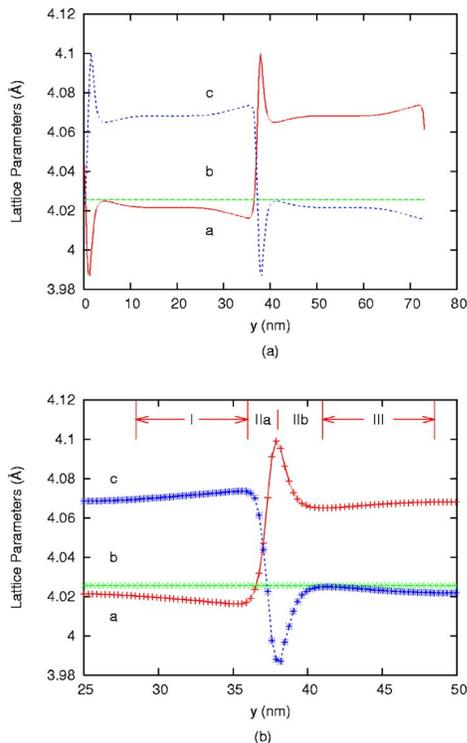
FIG. 2. (Color online) Unit cell distortions over the  $\text{BaTiO}_3$   $90^\circ$  domain wall. The polarization is along  $[0\bar{1}1]$  on the left and  $[0\bar{1}\bar{1}]$  on the right in the supercell coordinate system. (b) expands the domain wall region from (a). The relative magnitudes of (b) and (c) switch across the  $90^\circ$  domain wall, leading to an  $89.4^\circ$  rotation of lattice orientation.
