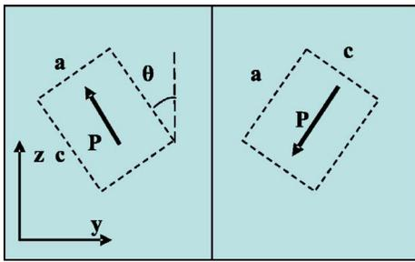
FIG. 1. (Color online) Supercell geometries used in the periodical boundary condition calculations. The polarization is along  $[0\bar{1}1]$  on the left and  $[0\bar{1}\bar{1}]$  on the right in the supercell coordinate system.
