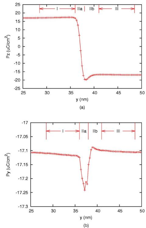
FIG. 3. (Color online) Polarization across the  $\text{BaTiO}_3$   $90^\circ$  domain wall. (b) and (c) show the  $P_z$  and  $P_y$  components in the amplified domain wall region from (a).  $P_z$  overshoots and then relaxes in the central layer.  $P_y$  increases its amplitude in the central layer.
