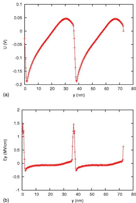
FIG. 4. (Color online) Electric potential (a) and electric field distribution (b). We find a large electric field (1.5 MV/cm) at the central layer (2 nm wide) of the domain wall, leading to 0.23 V electric potential change across the wall.
