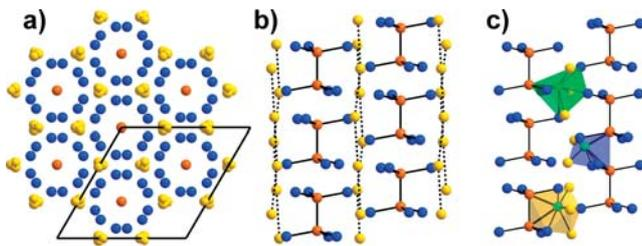
**Figure 1** (online colour at: [www.pss-rapid.com](http://www.pss-rapid.com)) Two views of the framework Zn<sub>12</sub>Sb<sub>10</sub> structure are shown looking along the rhombohedral [100] (a) and [110] (b) directions. Sb<sub>2</sub> atoms (orange) form dimers capped by Zn atoms (blue). Sb<sub>1</sub> chains (yellow) are not bonding. (c) The three distinct interstitial sites in the high temperature  $\beta$ -phase as defined in Ref. [2]: Zn2 (green), Zn3 (blue), and Zn4 (yellow) polyhedra.
