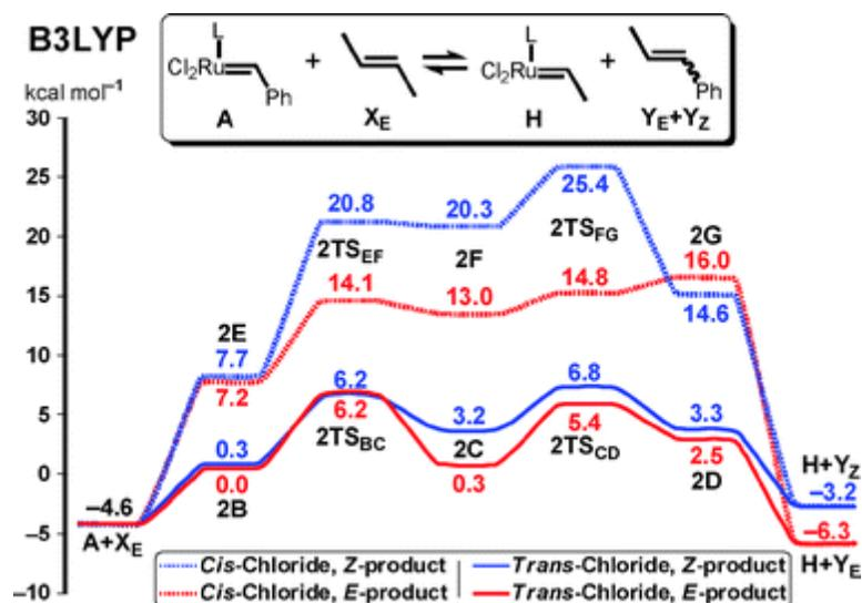
**Fig. 3** B3LYP computed energy profile ( $\Delta H$  in  $\text{CH}_2\text{Cl}_2$  at 298 K in  $\text{kcal mol}^{-1}$ ) for the bottom- and side-bound metathesis pathways for *E*-2-butene with Grubbs-II benzylidene catalyst.
