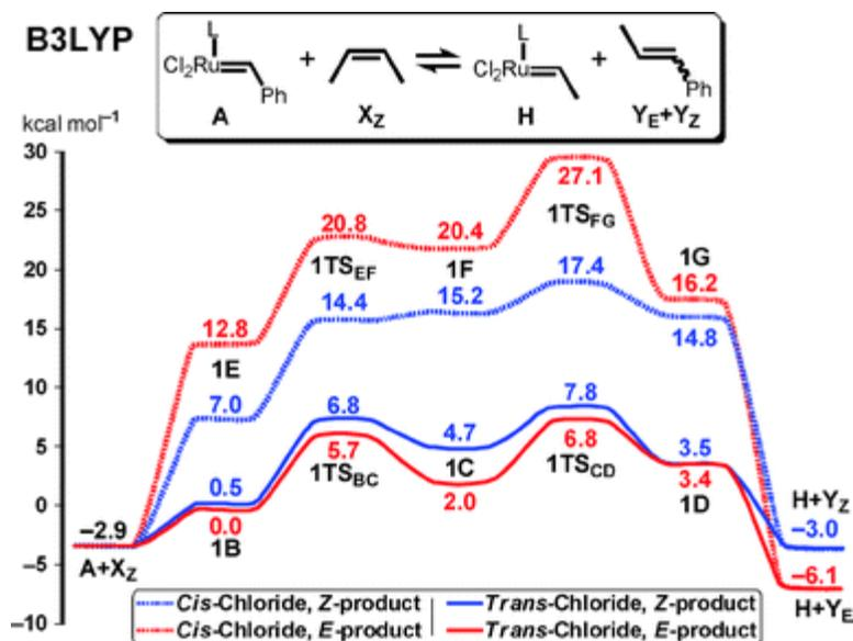
**Fig. 2** B3LYP computed energy profile ( $\Delta H$  in CH<sub>2</sub>Cl<sub>2</sub> at 298 K in kcal mol<sup>-1</sup>) for the bottom- and side-bound metathesis pathways for *Z*-2-butene with Grubbs-II benzylidene catalyst.
