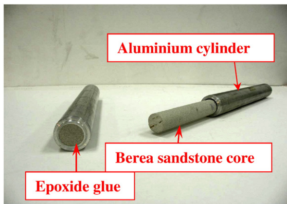
Fig. 7. Berea sandstone core preparation.
