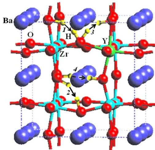
FIG. 1. (Color online) Proton transfer in BYZ. (1) Intra- $\text{ZrO}_6$ -octahedral proton transfer in the Zr–OH–Y configuration. (2) Intra- $\text{ZrO}_6$ -octahedral proton transfer in the Zr–OH–Zr configuration. (3) Intra- $\text{YO}_6$ -octahedral proton transfer. (4) Interoctahedral proton transfer between two neighboring  $\text{BO}_6$  octahedra.
