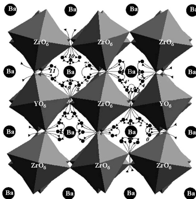
FIG. 2. Possible proton diffusion pathways in BYZ.
