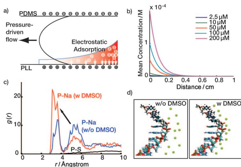
**Figure 2.** Electrostatic adsorption of DNAs on PLL surface and DMSO effect. a) The filling step. b) Simulation result of electrostatic adsorption of DNAs to PLL surface. c) Molecular simulation of the DMSO effect: the radial distribution function of P atom of the phosphate group and the sodium ions. The presence of DMSO pumps sodium ions from the 2nd shell to the 1st shell (arrow). d) Schematics for DMSO effect. Green circles represent sodium ions.
