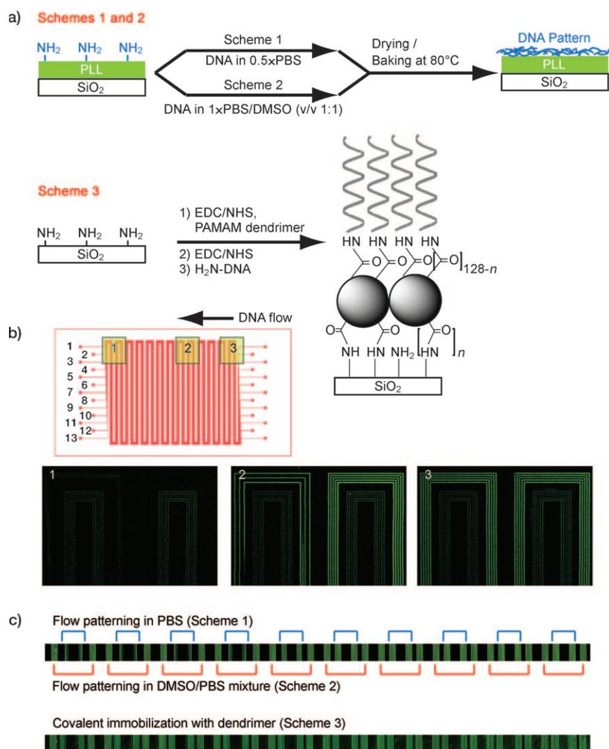
**Figure 1.** a) Surface treatment schemes. b) Design of the DNA patterning device (top) and fluorescence image of DNAs filled into the channel (still in solution). Outer five channels are filled with DNAs in 1:1 mixture of PBS and water (Scheme 1). The five inner are filled with DNA in a 1:1 mixture of PBS and DMSO (Scheme 2). Three channels in between are left empty for visualization. c) Fluorescence images of patterned DNAs by three schemes.
