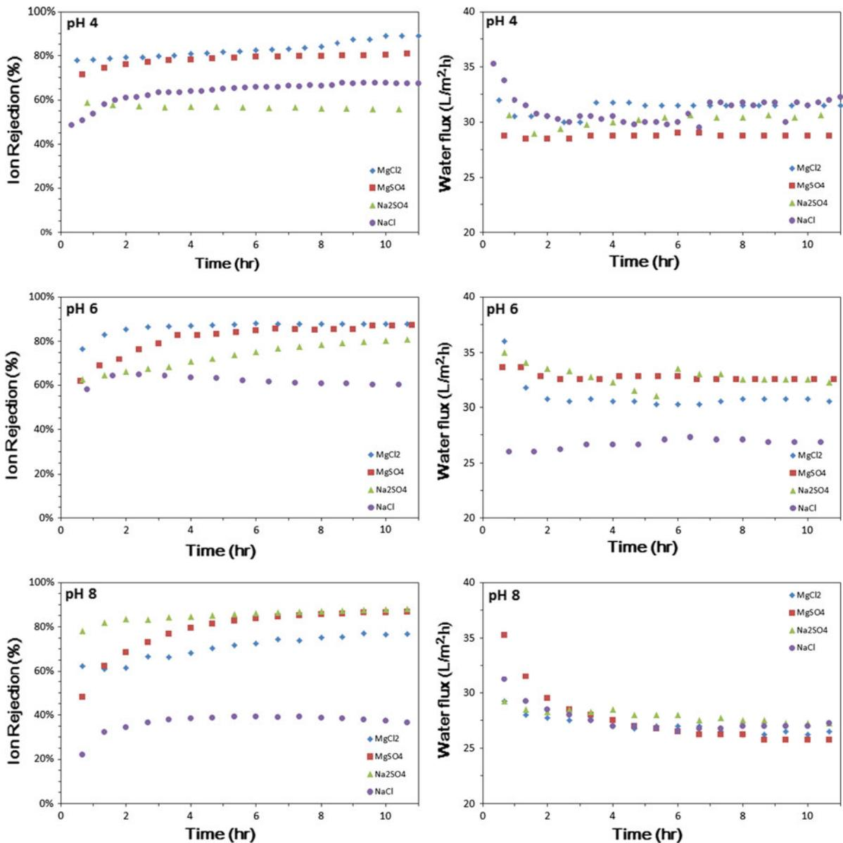
**Fig. 6** Ion rejection and water flux of NFC–PEI-1 at pH 4, 6, and 8 as a function of time at room temperature. A cross-flow filtration system was utilized to measure the ion rejection and permeate flux of the membrane
