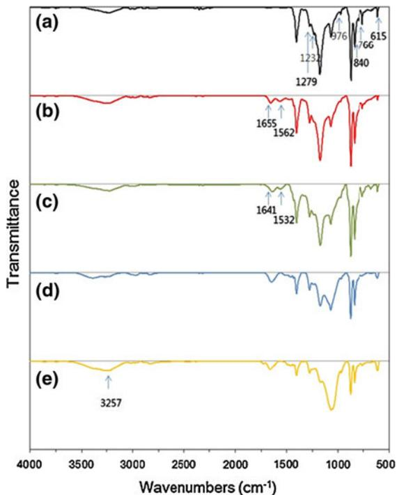
**Fig. 4** FTIR-ATR spectra of a PVDF microporous support (a), a PVDF + PEI nanofibrous scaffold (b), NFC-PVDF-PEI-1 membrane crosslinked with trimeosyl chloride (c), NFC-PVDF-PEI-2 membrane crosslinked with 1-3 dibromopropane (d), and NFC-PVDF-PEI-3 membrane crosslinked with epichlorohydrin (e)
